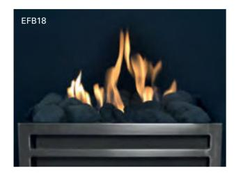
The EFB18 fits a wide selection of Chesneys fire baskets. The fire features a slider mechanism that allows the amount of heat being generated to be regulated. The EFB18 is available with a choice of logs, coals or pebbles. It has a 5 litre fuel reservoir with a heat output of 3.5 kilowatt and burn time of approximately 7½ hours.
